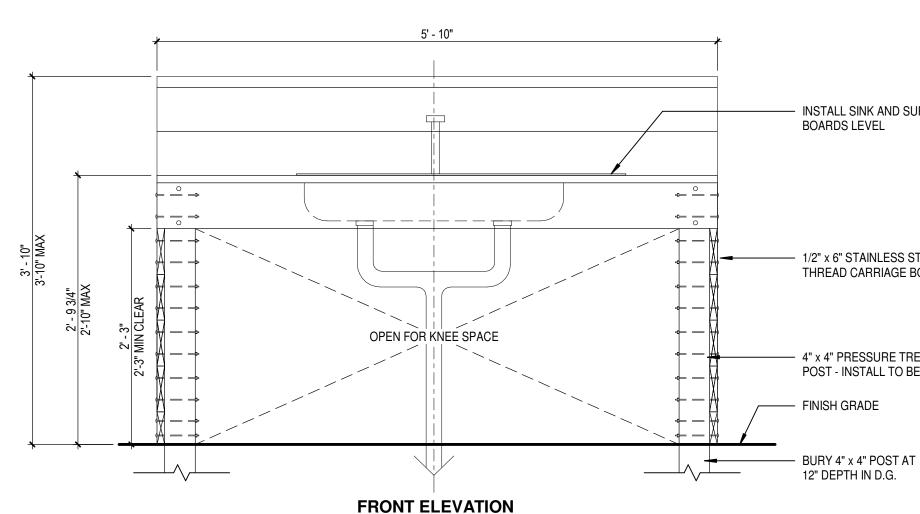
2. CONTRACTOR SHALL PROVIDE SHOP DRAWINGS FOR REVIEW AND APPROVAL PRIOR TO FABRICATION. 34 WORK TABLE AND SINK DETAIL
